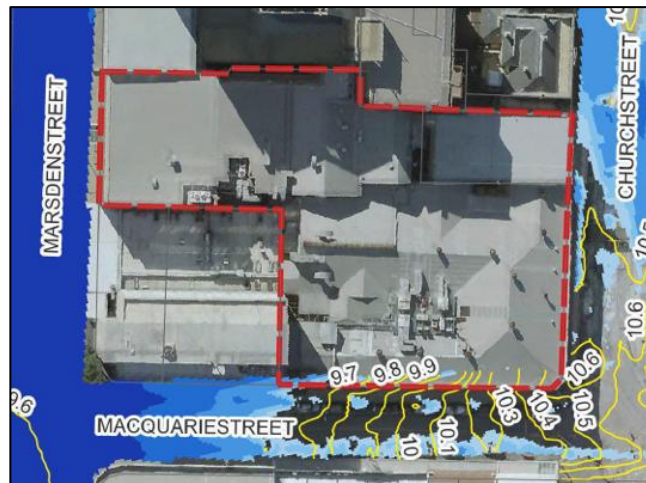
Figure 25: Council's 1% AEP river flood modelling Figure 26: Applicants 1% AEP overland flow modelling
